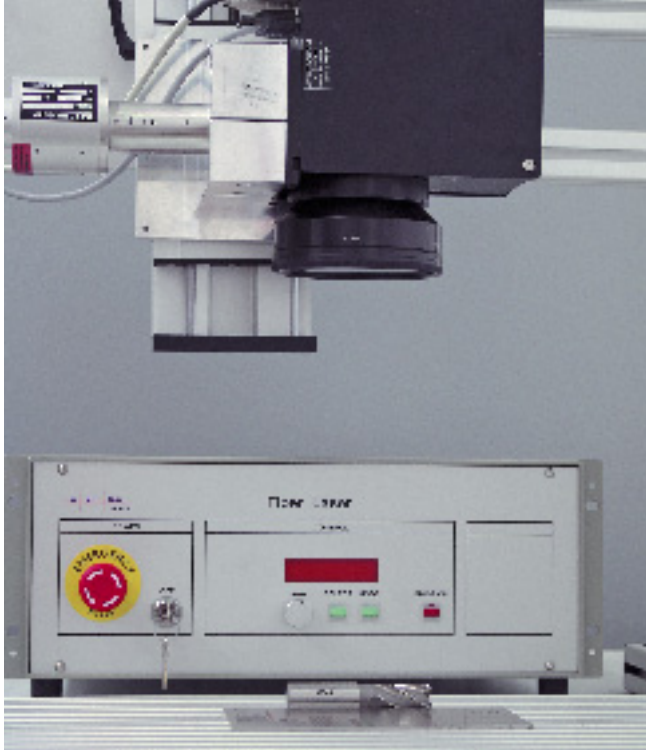
YLR-200-SM laser integrated with a scanner in an engraving machine
