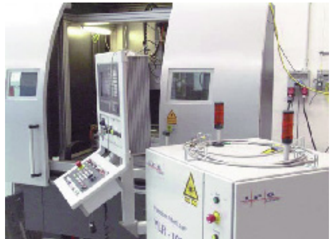
YLR-1000-SM 1kW fiber laser integrated in a cutting cell
