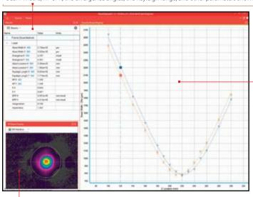
This window presents measurements of beam width vs. position for a given run. After measuring a few points, the software extrapolates a curve fit. The Xs and Ys represent individual measurement points. The solid lines present the best fit hyperbola of the beam propagation equation to the measured points. The M² and other laser parameters are computed from the best fit hyperbola since it provides a smoothing of the data points.
