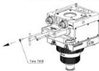
Step 6 Pull lens module into exchange holder using the key Remove exchange holder from head
